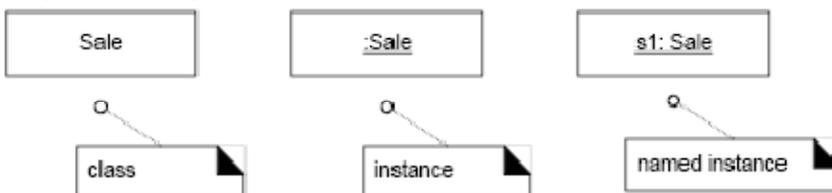
Fig: Class and corresponding object(instance) notation
